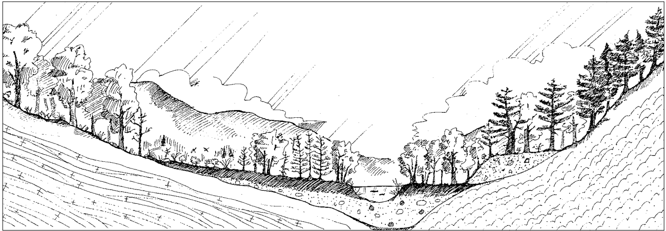
Fig. 1-1 This cross section of a landscape in the Vermont Valley shows that bedrock (straight or wavy lines) underlies everything, but in some places the surficial deposits (pebbly gravel and dark-hatched peat) cover the bedrock and have a greater influence on the vegetation. (Source: Darien McElwain, “Wetland, Woodland, Wildland”)
