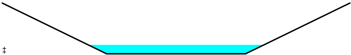
Figure B-1. HydroCAD summary of a grass channel during the water quality storm event.
