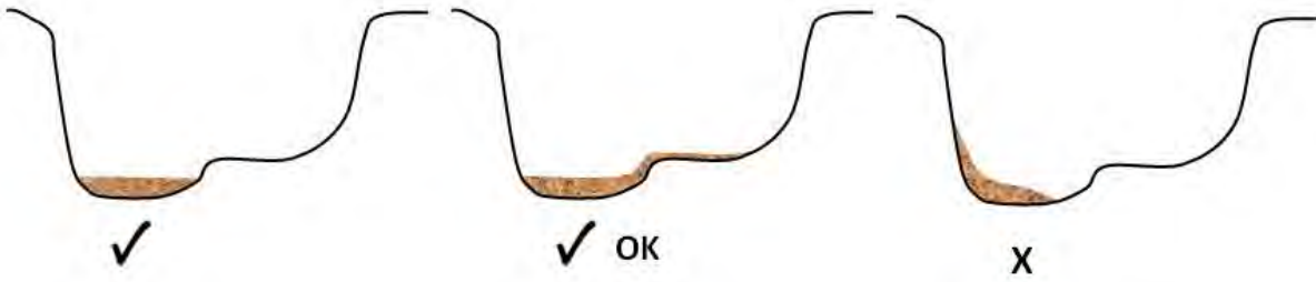
Figure 5.3-2: Schematic of reinstatement of native bed materials including preferred (left), acceptable (middle), and incorrect (right).
