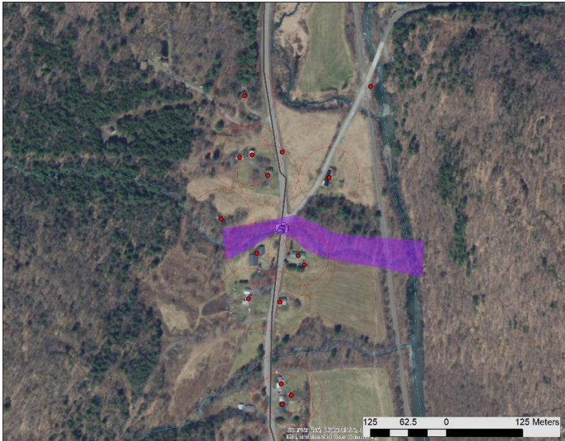
Figure 5. 50m buffers were created around all residences within 300m of a transportation structure and overlaid with the movement pathway polygon (Site 12a-10, Braintree).
