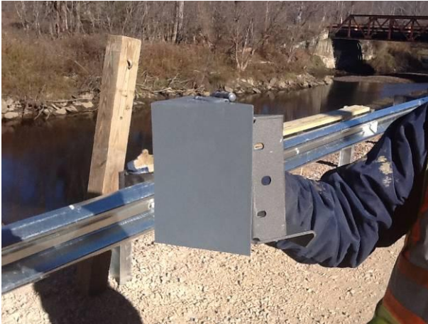
Fabricated housing for angling camera to the side
