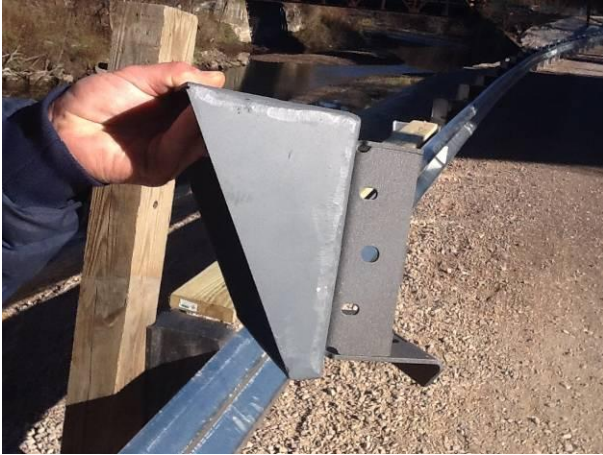
Fabricated housing for angling camera down
