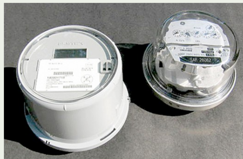
Digital smart meter (left) as compared to a traditional analog meter (right) Source: www.CaliforniaPhoton.com
