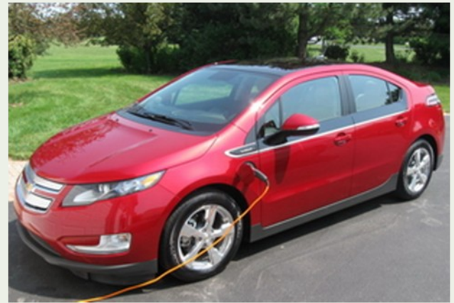
The Chevrolet Volt is a plug-in electric vehicle with a conventional engine designed to extend the range of first generation lithium ion automotive battery. Source: www.CleanMPG.com
